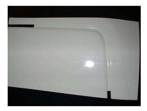
Illustration of a completed recess corner. Some material has been removed from the recess for clarity.
