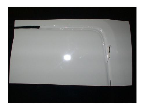
• Apply VWS to the flat panels and cut to overlap the edges of the vinyl in the recesses. Use gentle heat if necessary on the corners. This application method hides the joint line from view and ensures that the vinyl remains in the recesses.
